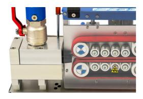
**BDJ** Max is a professional cable blowing machine designed for blowing cables within 6-15mm range into ducts diameters: 32, 40 and 50mm. Solid and simple construction ensures easy operation and longevity of the unit. Machine blows cables with 110 m/min speed. Achievable distance is 2500 m. The unit can be upgraded with an **extra blowing** head for extending the blowing range of BDJ Standard with cables Ø 2,5 mm – 10 mm and microducts Ø 5 mm – 16 mm.
